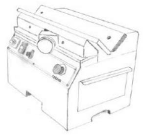
Bevelling - polishing machine to obtain bevels from 1 to 10 mm. Working angle 45°
